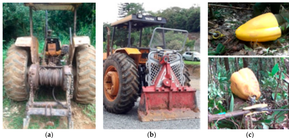
Figure 1. Harvesting equipment used: (a) Standard 2 × 2 farm tractor with a TMO Caçador ® winch used in the conventional method (CM); (b) TAJFUN ® winch fitted on a 4 × 4-farm tractor used in the alternative method (AM); (c) Skidding cone and snatch block supplementing the AM extraction.
